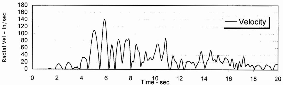
Figure 6 Energy time history and corresponding relative radial displacement and velocity time histories at Pier 9 (Ground motion set #2)
