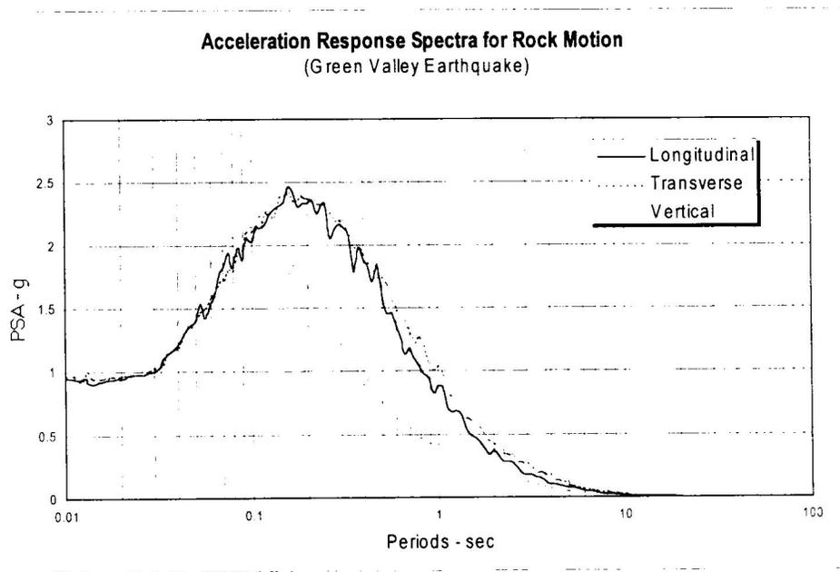
Figure 2 Rock motions spectra of Green Valley earthquake
