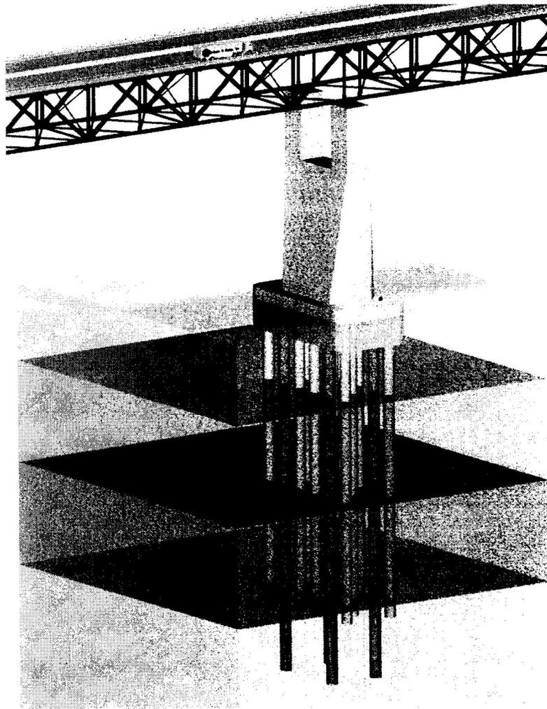
Figure 1 Schematic 3D view of typical pier and pile group foundation
