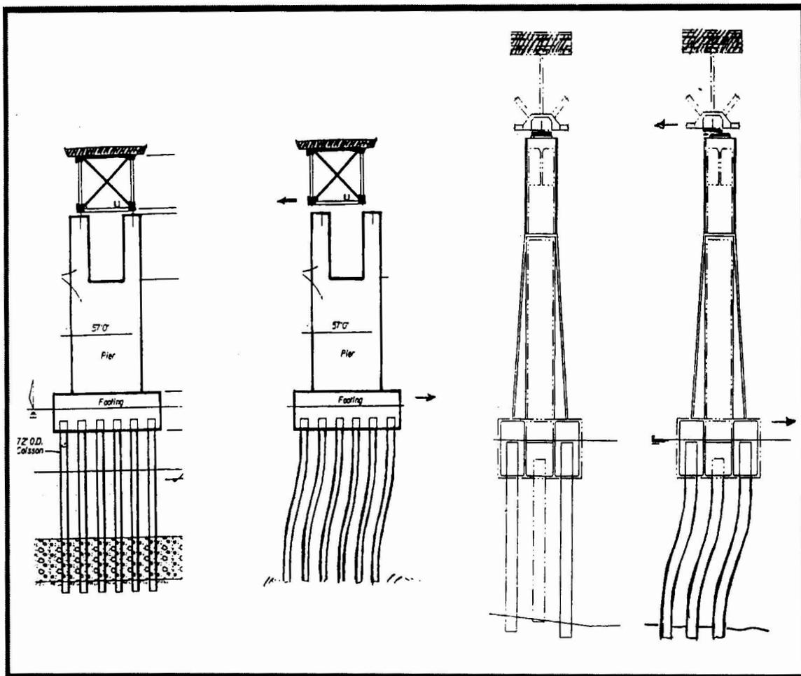
Figure 4 Dynamic behavior of isolation bearings at typical pier
